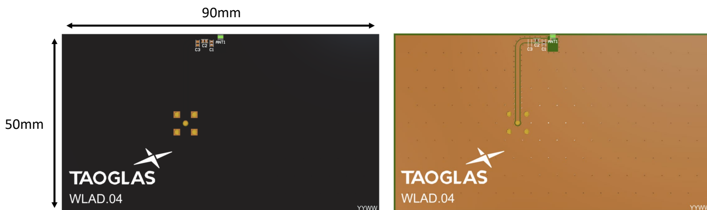
Top Side (WLA.04 placement on 90x50mm PCB)
