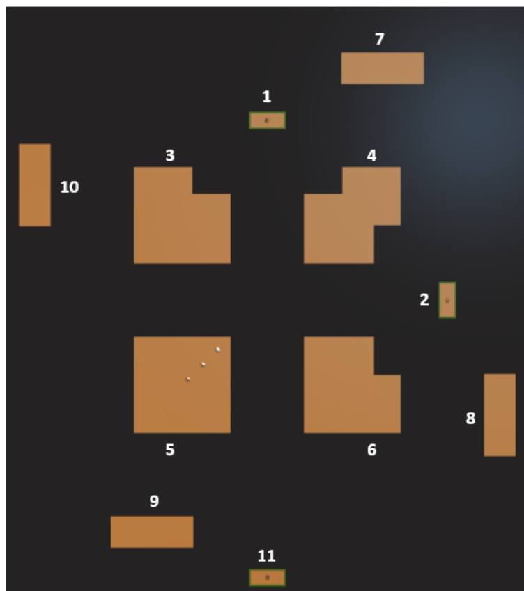
3D Top View image of the exposed solder mask for the HP5354.A
